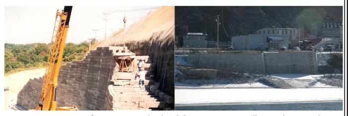
Precast Concrete system for use in Streambanks, Slide correction, Seawalls, Cut slopes, Explosion Barricades, and all variety of grade separation applications where a single wall or bin wall is best. Walls withstand high flow rates and submersion with rapid draw-down. Ideal for riverside use. Architectural stone pattern facing also available. PennDOT approved.
